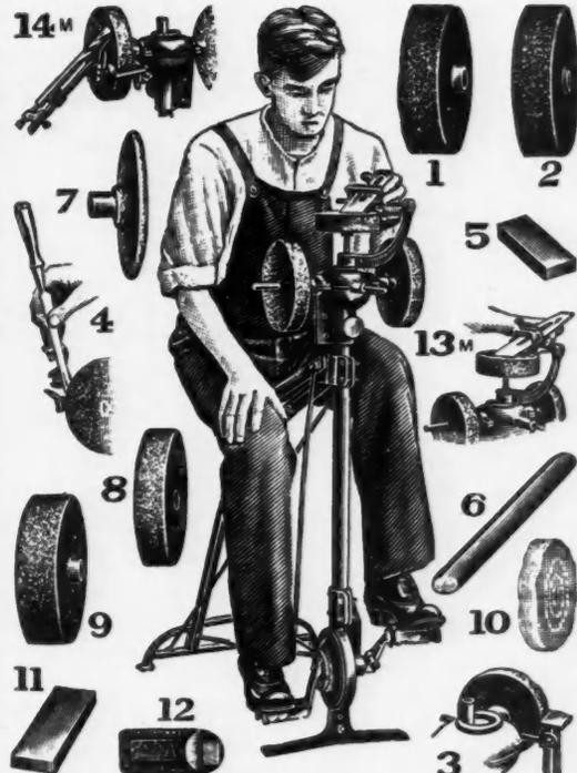
FOURTEEN MACHINES IN ONE. 1—Fine Dimo-Grit Wheel. 2—Coarse Dimo-Grit Wheel. 3—Universal tool rest. 4—Chisel and plane bit guide. 5—Dimo-Grit razor hone. 6—Dimo-Grit scythe stone. 7—Dimo-Grit saw gummer. 8—Felt polishing wheel. 9—Medium Dimo-Grit Wheel. 10—Cloth Buffing wheel. 11—Dimo-Grit oil stone. 12—Dimo-Grit pocket hone. 13M—Plane bit honing attachment. 14M—Twist drill sharpening attachment.
