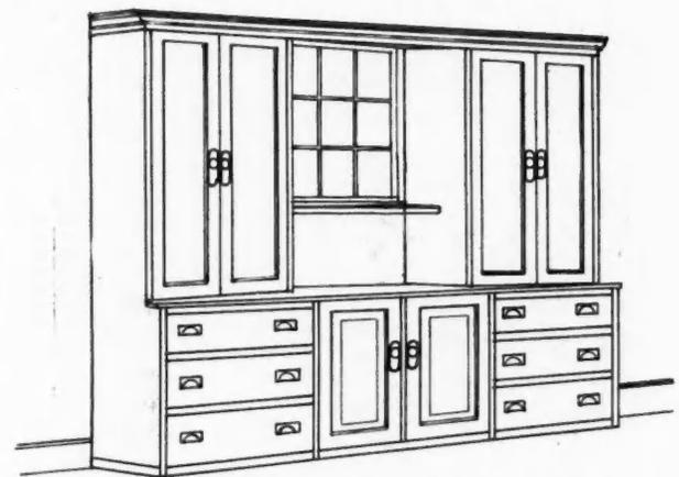
Fig. 2. Large Kitchen Cupboard, Lighted at Center by Casement Window
