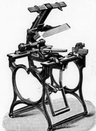
**Machine for Trimming and Punching Slate**
