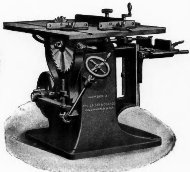
Fig. 5. No. 3 Improved Variety Saw (With Boring Attachment)
