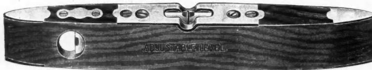
Dimensions—9 in. long,  $1\frac{1}{4}$  in. deep,  $\frac{3}{8}$  in. thick in center, tapering ends, made of rosewood highly polished, tips top and bottom inlaid with brass. Accurately tested bottles well protected.
