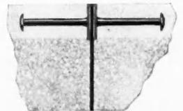
Vertical Section through Plate-Protected Joint
