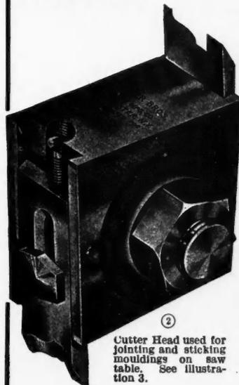
Cutter Head used for jointing and sticking moldings on saw table. See illustration 3.
