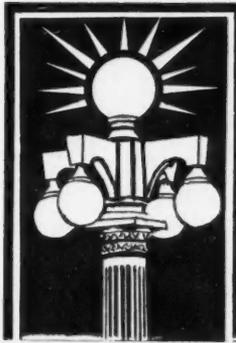
These reinforced concrete standards are handsome, durable, artistic and inexpensive. They do not rust like cast iron, become dented like sheet metal, or rot like wood. They require neither painting nor repairs, and are not affected by weather conditions.
