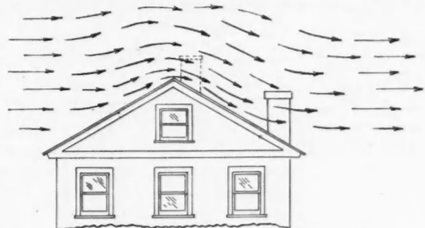
Fig. 5. Effect of Sloped Roof on Chimney Draft
