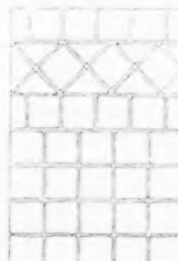
By breaking joints in one course, the border is made wide
