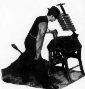
One Throw of the Lever Delivers Eight Brick on each side of the machine
