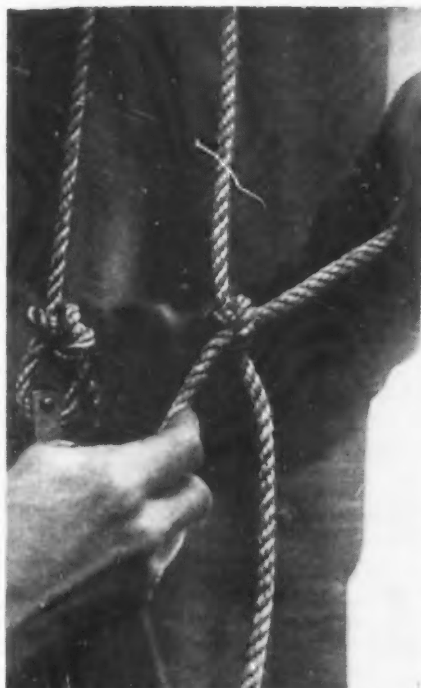
Fig. 2. Safety rope is tied around control line with two half-hitches.
