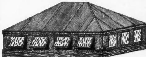
with swinging sash. Sides 24" high; all windows on each side made to open at the same time. Operating device securely locks them open or closed.
