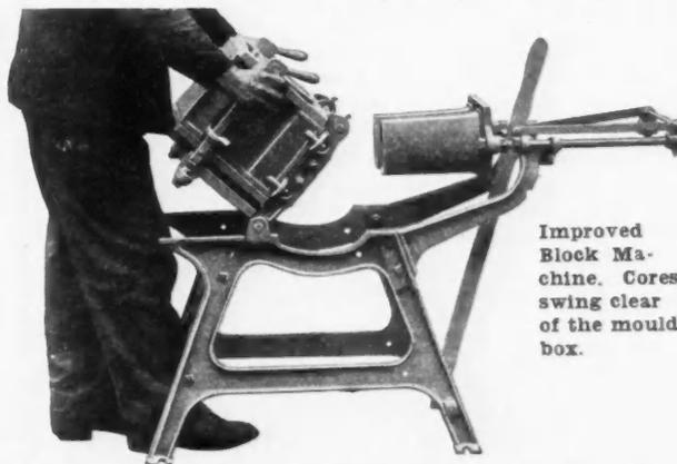
Improved Block Machine. Cores swing clear of the mould box.
