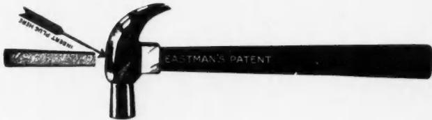
handle will never loosen. It is keyed from the outer end with a wooden plug driven through the eye into the handle. Because of its special construction, the handle acts as a shock absorber and prevents jarring of the hand.
