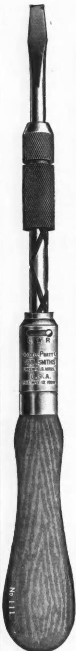
This Screw Driver is made stronger and heavier than most tools of this character so that it will drive large screws into hard wood. The slant angle of the spiral is 20°, giving more power than the ordinary tool of this type. It can be used as right or left hand, automatic or ratchet, or by moving the shifter to the star on the nickel-plated shell, it can be used as a plain screw driver.
