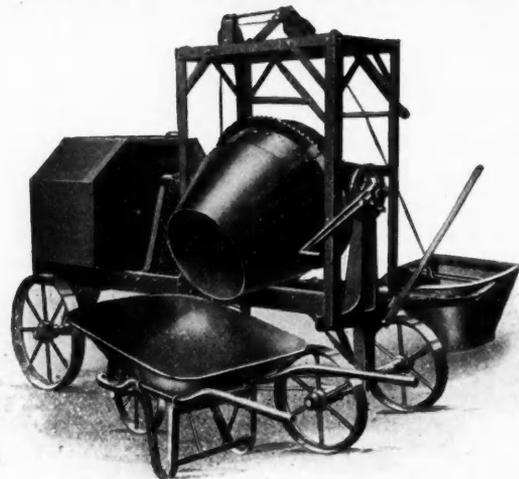
At a small additional cost we will equip the Winner-Four with power side-loader, increasing the capacity about one-half because you can prepare one batch while you mix the other. The above photograph tells the story and the price is \$240.00.
