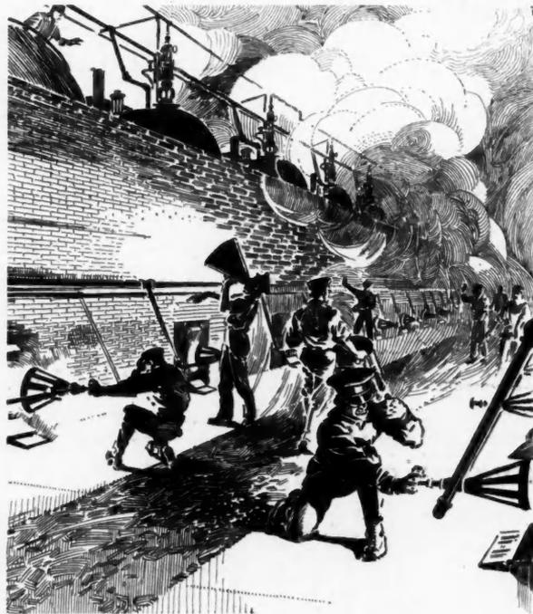
Melting Pure Asphalt at a Temperature of 290° Fahrenheit. Scene in Factory of The Heppes Co., Kilbourne Ave. and Fillmore St., Chicago, manufacturers of Flex-A-Tile Asphalt Shingles, Utility Wall Board and Asphalt Paper.
