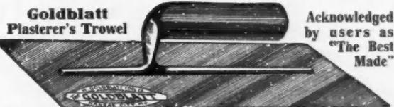
No. 1G—Finishing Trowel, made of 22 or 24 gauge **best trowel steel**, highly polished and etched. Mounting extends within one inch of each end of blade and has **ten large rivets**. Has plenty of spring. Lime cannot work between blade and mounting. Three sizes, 4 1/2 x 11 inch, 4 3/4 x 11 1/2 inch, 5 x 12 inch. Low, medium and high mounts. Price \$2.00 charges prepaid. Your dealer or direct.
