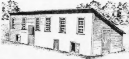
Shed Roof Permanent Hog House —When only ten or twelve brood sows are kept and a central house is preferred, a building 16 by 48 feet will prove useful. Cement floors can be constructed to good advantage in front or at the rear. For farrowing 12 separate pens can be obtained by putting in a temporary partition lengthwise and dividing the space on each side equally.
