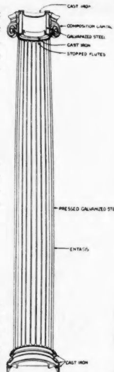
Construction of Union Metal Column.
