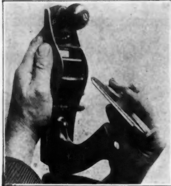
Plane Has Instant Setting Screw.
