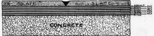
Showing Approved Construction for Flat Steel Roof Over Concrete.
