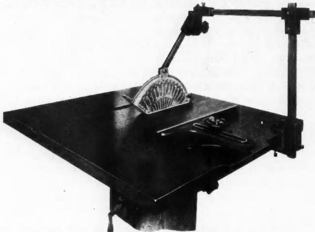
Safety Guard for Buzz Saws—Will Fit Any Machine.
