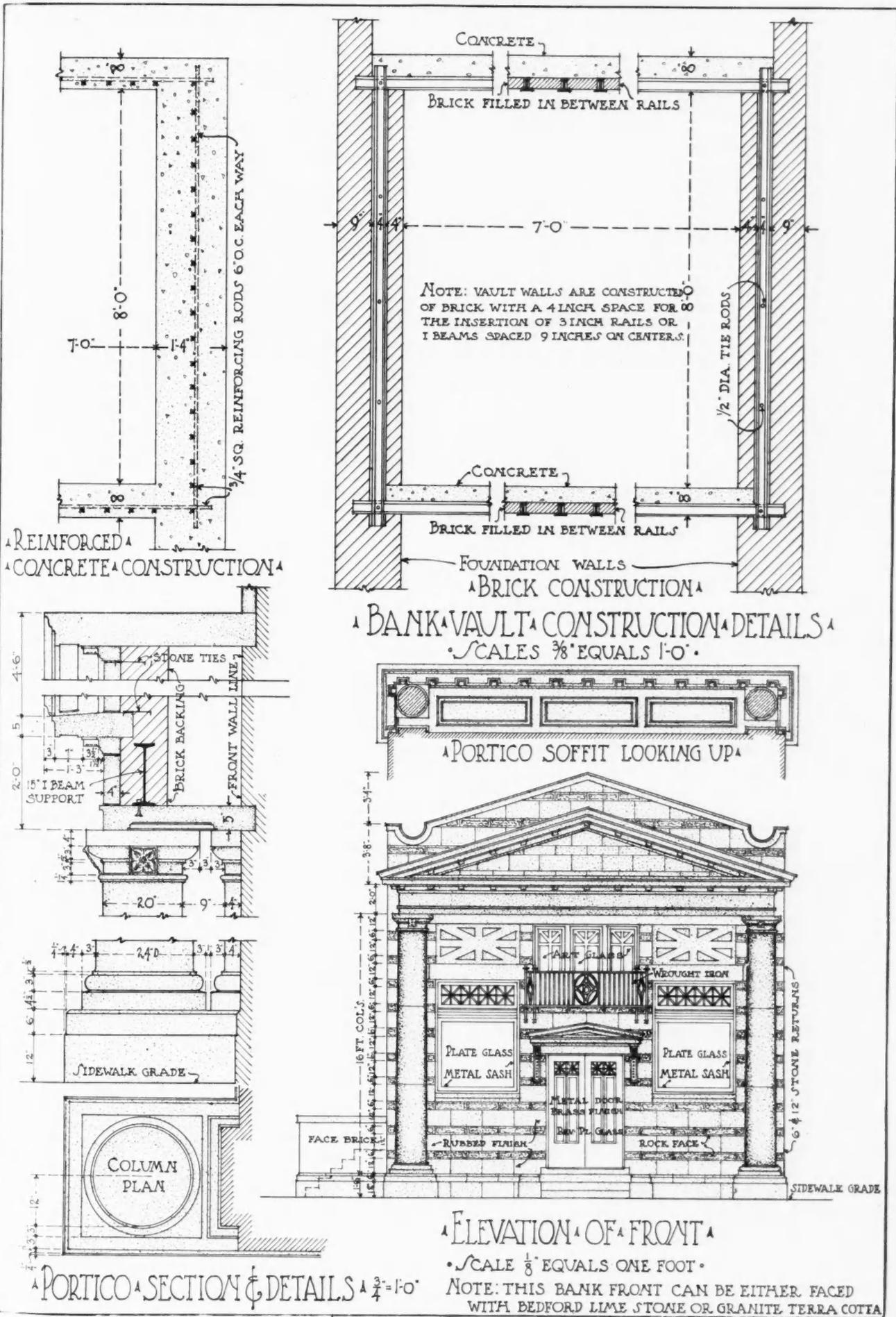
Details of Bank Front; also Details of Two Methods of Construction for the Fireproof Vault (Design No. 6748, Illustrated on Page 54.
