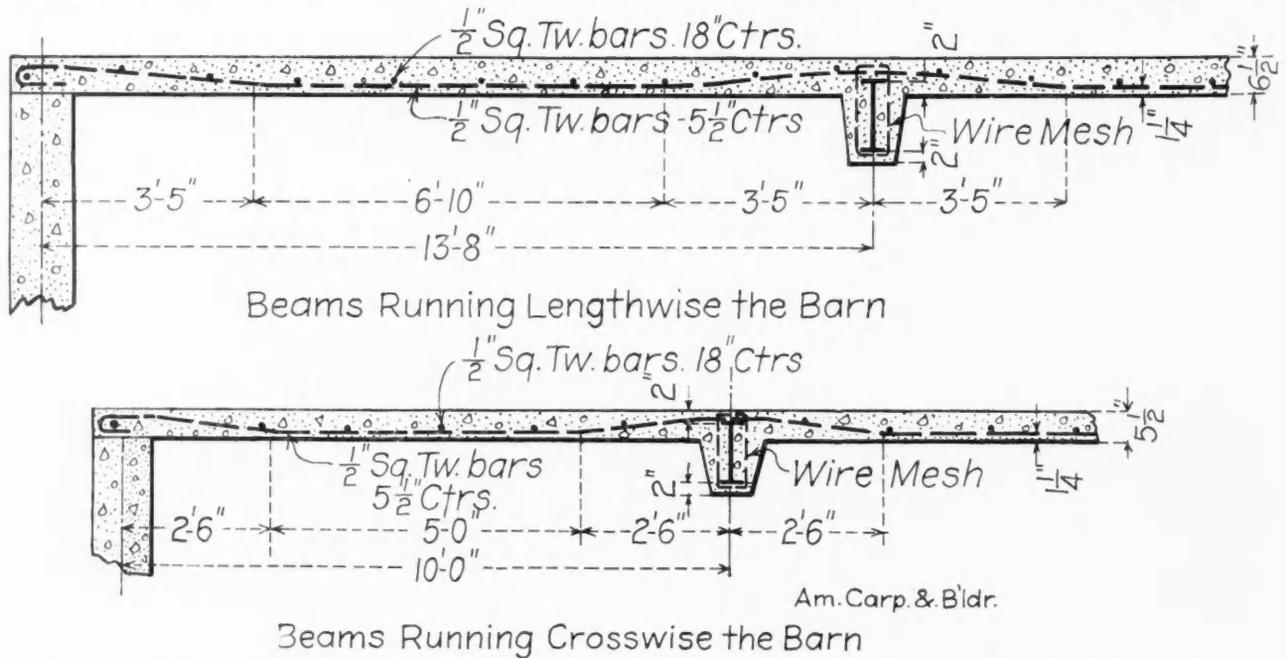
Details of Beams and Floor Slabs (Figured for the Two Optional Ways of Running the Floor Beams) Showing Reinforcing as Placed Under Hay Mow.
