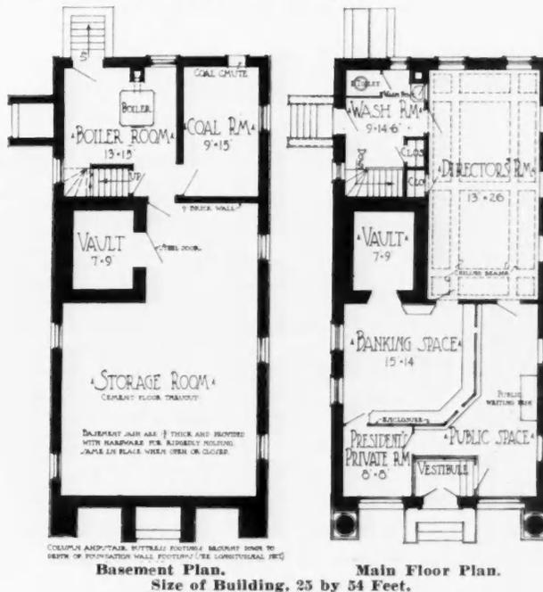
Basement Plan. Main Floor Plan. Size of Building, 25 by 54 Feet.
