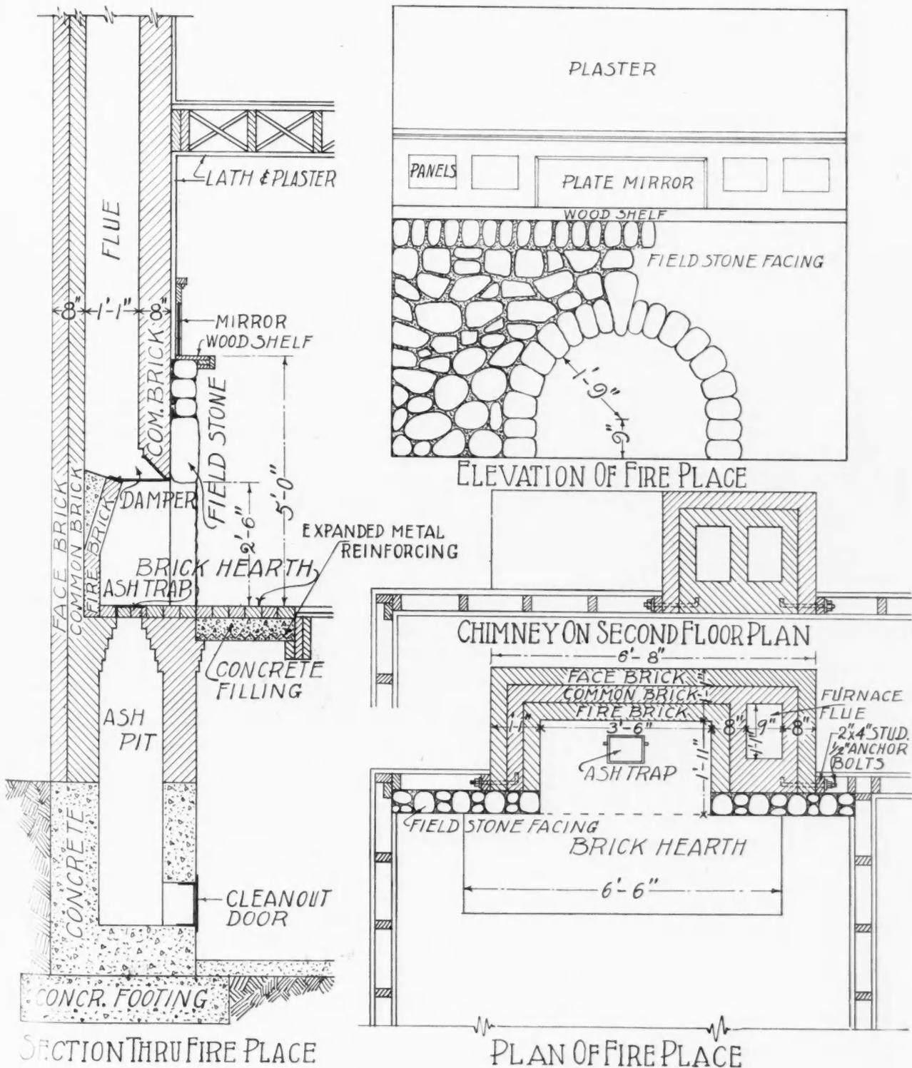
Details of Construction of Fireplace Built with Field Stone Face.
