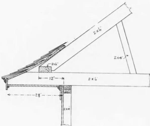
Cornice Detail for Roof with Slight Curve at Eaves.
