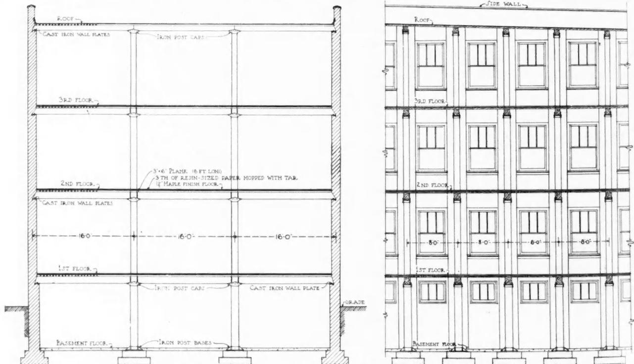
Fig. 71. Two Views of Wooden Mill Construction Type of Commercial Building.
