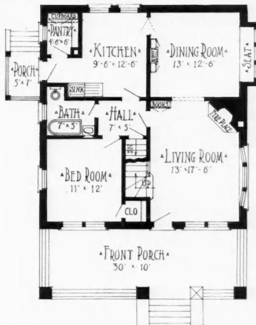
Floor Plan and Arrangement of House, 30 by 32 Feet, Built by J. V. Allen.
