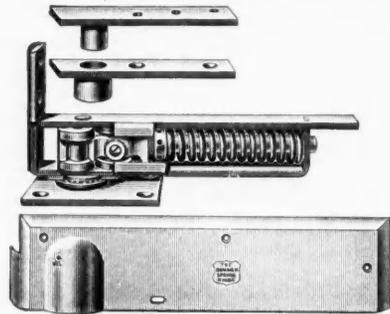
The most durable hinge of its type; holds the door open when swung to 90 degrees at either side. The spring-action can also be entirely released as long as desired so that the door will swing free, without spring-action, in either direction, by inserting a wire nail (when the door is open) into a hole provided in the side plates for that purpose. The spring-action can be restored by withdrawing the nail.
