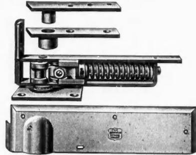
The most durable hinge of its type; holds the door open when swung to 90 degrees at either side. The spring-action can also be entirely released as long as desired so that the door will swing free, without spring-action, in either direction, by inserting a wire nail (when the door is open) into a hole provided in the side plates for that purpose. The spring-action can be restored by withdrawing the nail.
