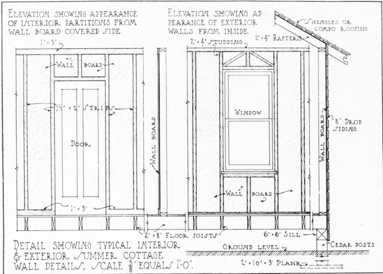
Details of Construction and Inside Finish Using Wall Board. The Wall Board is Nailed to the Outside of the Studs which are Dressed Four Sides, Stained, and Serve as Panel Strips, Making a Very Attractive Camp Interior. Drop Siding or Rough Inch Boards are Nailed on Over the Wall Board for the Exterior Siding. Inside Partitions Constructed of Wall Board and Light Panel Strips.
