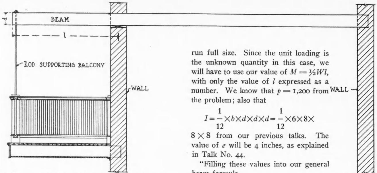
Fig. 4B. Cantilever Beam with a Single Load at End.
