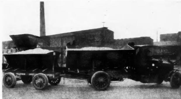
Heavy Trailer with Special Side Dumping Body for Handling Sand and Crushed Stone.
