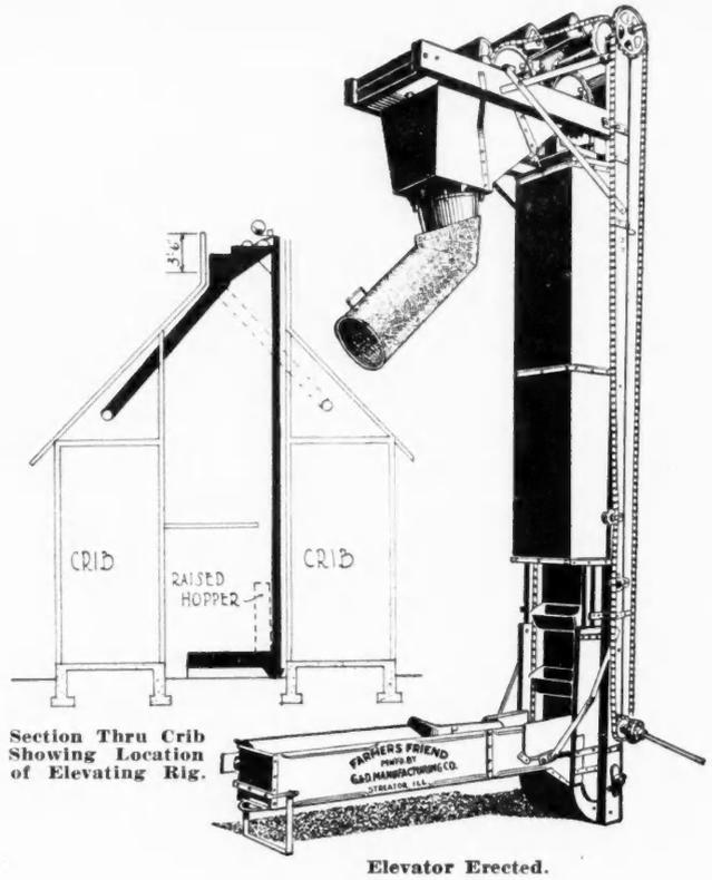
Section Thru Crib Showing Location of Elevating Rig.
