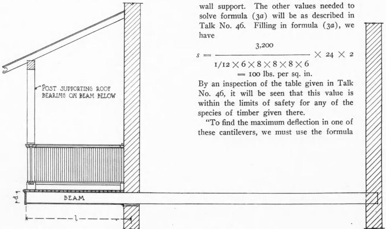
Fig. 4C. Cantilever with a Combination of Uniform Load and Concentrated Load.
