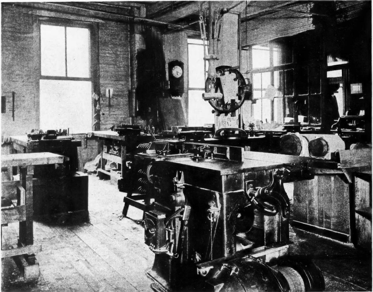
Saw Table and Work Benches. Each Bench is Equipped with a Little Electric Power Bench Planer. Note Lighted Office Partitions Giving Clear View of Shop.
