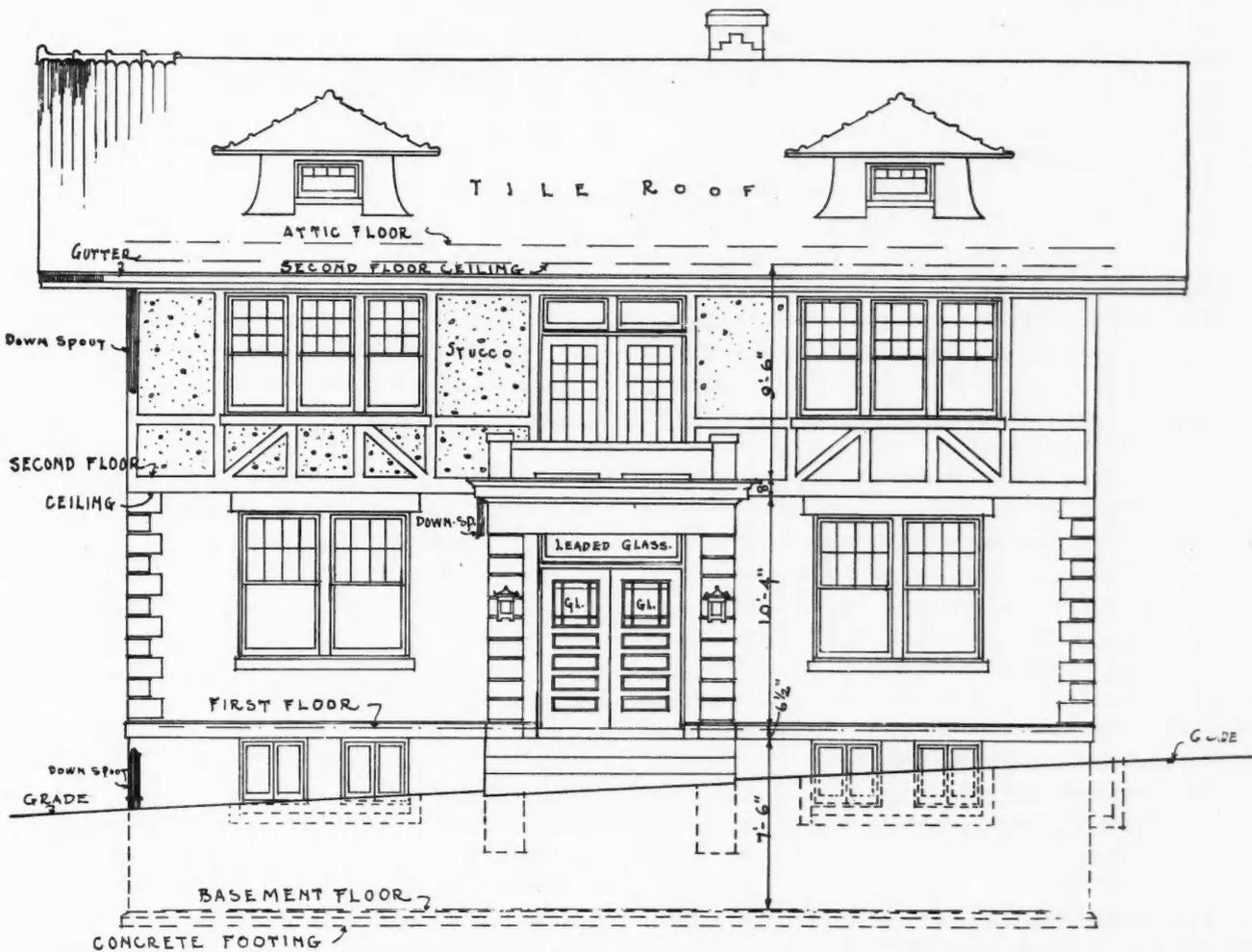
Front Elevation and Photograph of New Office Building of Sparks Milling Company, Alton, Ill., Designed in Swiss Chalet Style, Stone and Cement Plaster Construction, Pfeifferberger & Son, of Alton, Architects.
