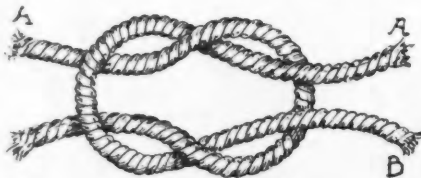
Square Knot if A A is Standing Part of Rope.
