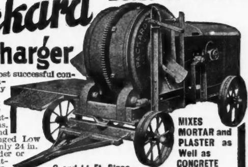
The choice of the most successful contractors. A high speed, high-efficiency mixer especially made for fast work on stiff concrete for Curbs, Sidewalk, Gutters and Foundations. Light, Strong and Durable. Has Hinged Loading Platform only 24 in. high. Power Loader or Batch Hopper if wanted. Sold with our "Money-Back" Guarantee—cash or easy payments—price astonishingly low. Prompt delivery from stock carried in all large cities. Write for catalog today.
