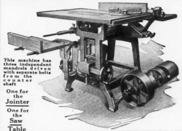
This machine has three independent mandrels driven with separate belts from the counter shaft
