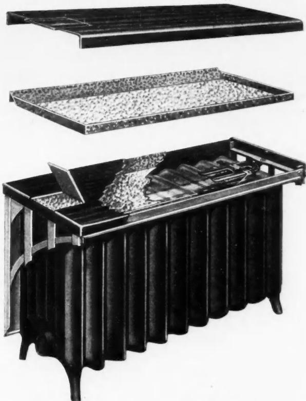
Perspective Detail Showing Parts and Indicating Strength of Humidifier, Which Also Serves as Shelf or Seat.
