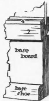
Upper Detail Shows How Moulding Numbered 2 Forms Connection Between Wall Board and Baseboard. Lower Detail Shows How Moulding Numbered 2 May be Used as Door Casing and Also How It Is Used in Connection with Regular Casing.
