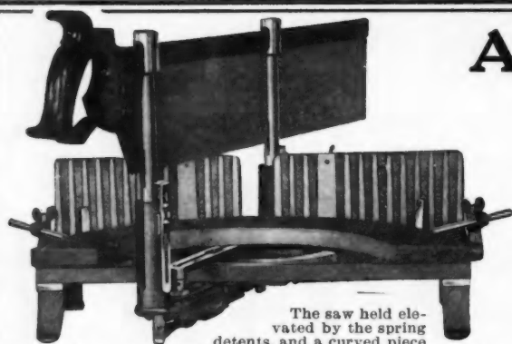
Fig. No. 4 The saw held elevated by the spring detents, and a curved piece of stock held in position by the length gauges.
