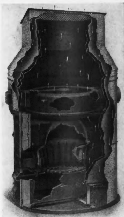
Cross-Section Showing How Cold Air Returns and Is Heated Again in a Pipeless Furnace.
