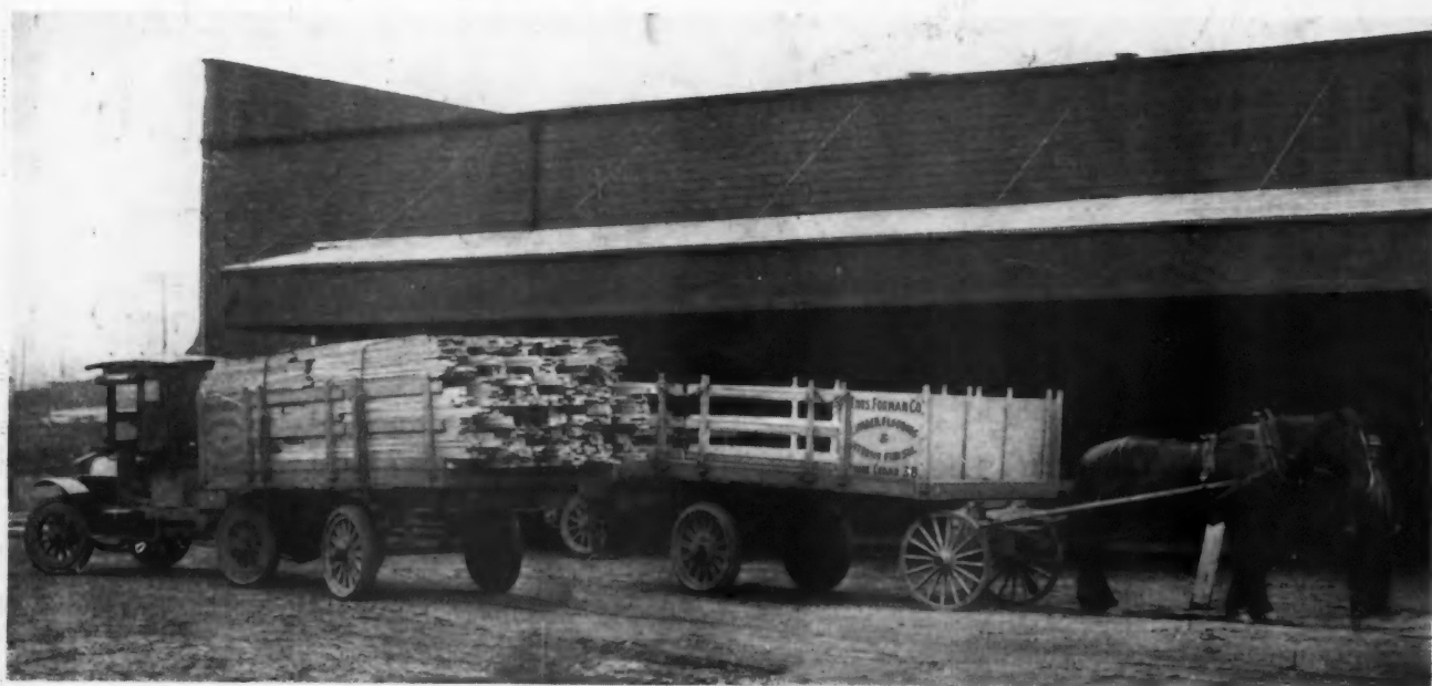
The Thomas Forman Co. Operates Two Semi-Trallers in Connection with Its Ton-and-a-Half "Federal" Truck. Note the One-Horse Dolly That Is Used to Haul the Semi-Traller About the Yard.
