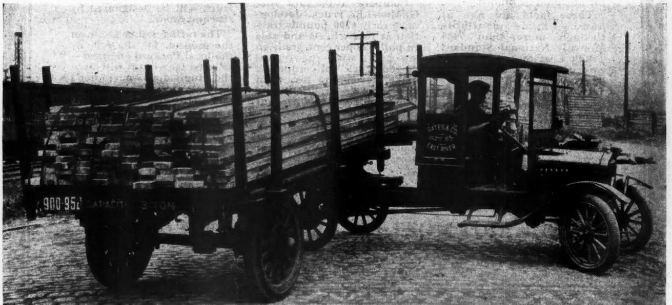
This Picture Shows the Adaptability of the Trailer for Making Short Turns in the Lumber Yard. This "Trailmobile" Is One of Several Owned by Church E. Gates & Co., New York City. The Jack-Knife Frame Enables the Driver to Dump the Lumber in a Few Minutes.
