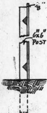
Fig. 1. Side Elevation of Rail Which Has Been Ripped Diagonally to Save Lumber.
