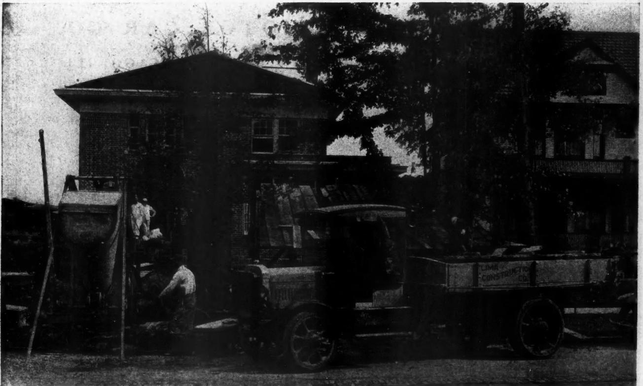
Three and One-Half Ton "Gramm-Bernstein" Truck with Special Square Cornered Dump Body to Speed Up Loading of Brick, Owned by the Lima Construction Co., Lima, Ohio. The Side Boards Are Removable to Form Platform Body When Hauling the Concrete Mixer or Other Heavy Machinery.
