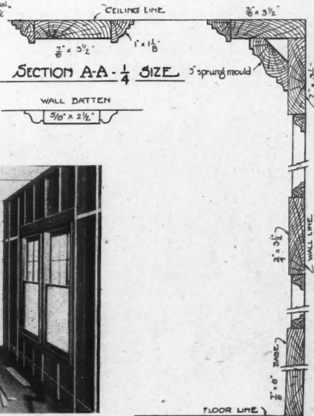
List does not include door and window casings nor baseboard. Wall panel moulds to be used along top of baseboard but not around door and window casings.
