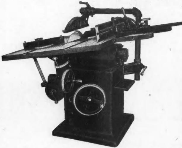
Direct Motor Driven Variety Saw Bench Designed to Save Floor Space and Eliminate Belt Hangers and Loose Pulleys. It Runs on 220-Volt Current.
