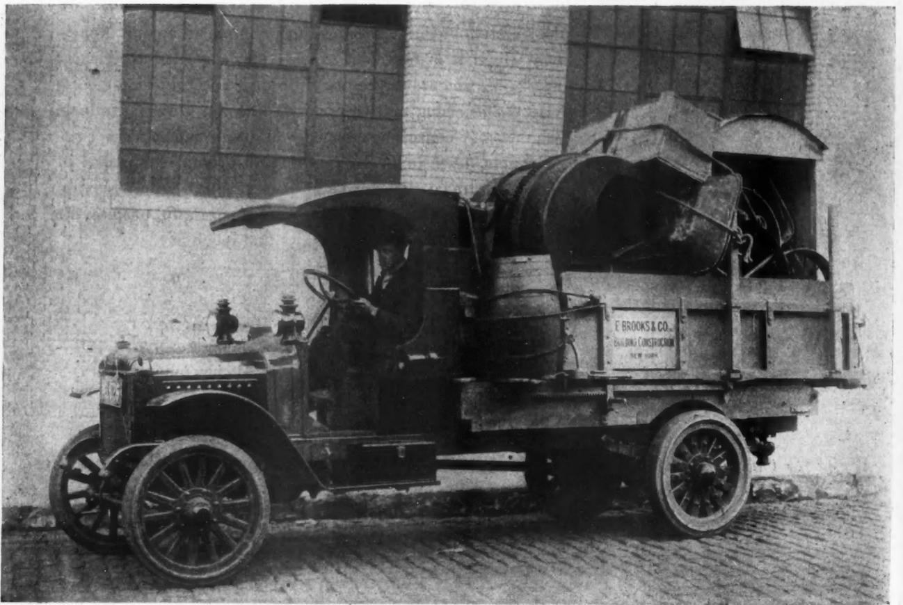
E. Brooks & Co. Are Progressive Contractors in New York City. They Use the Latest Machinery and Equipment on the Job and Motor Trucks to Get Them There. Here Is a Typical Load of Construction Machinery on Its Way to a New Contract. Consider the Time Saved by This Method of Transportation. This One-Ton "Republic" Loses No Time Getting There.
