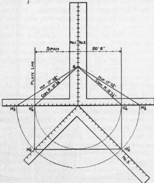
Fig. 1. Three Squares Placed so as to Represent Run and Rise of the Common Rafter and Corresponding Hip.
