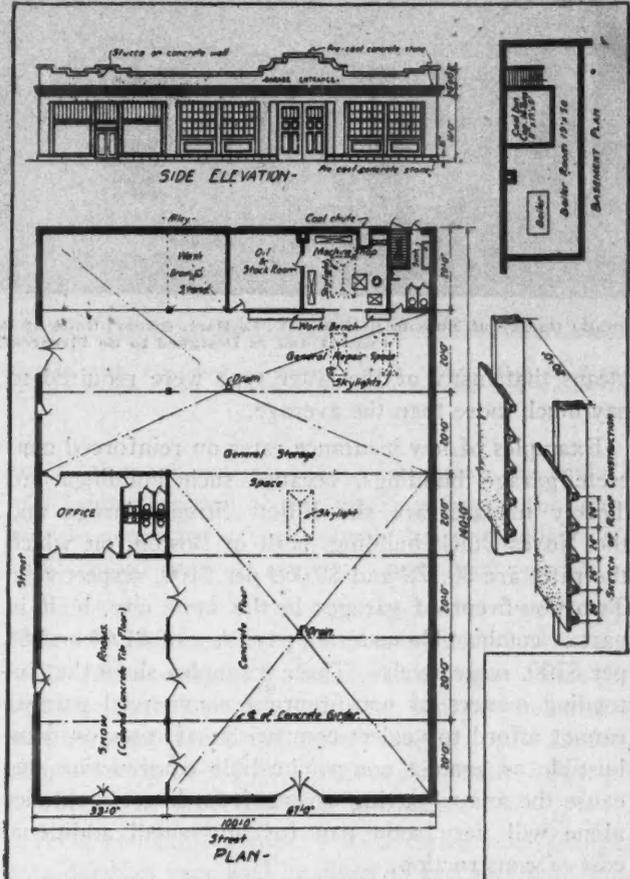
Model Floor Plan and Construction Details for Combination Public Garage and Show Rooms. The Building is Stucco with Pre-Cast Concrete Stone Trim, 100 Feet Wide and 140 Feet Long.
