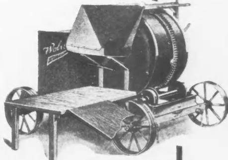
Wolverine half-bag capacity low charger—equipped with 3 HP horizontal gasoline engine with magneto—engine housing—power loader—measuring tank—sells for \$325.00, f. o. b. factory. May be equipped with batch hopper.
