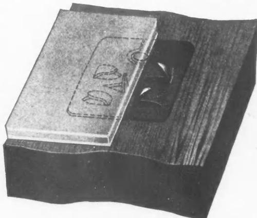
**Dotted Lines Show How Curved Prongs Clinch as They Are Forced Into Wallboard. Straight Center Prong Keeps Board From Slipping to Either Side. Prongs on the Right Show Normal Position Before Board Is Applied to Fasteners.**
