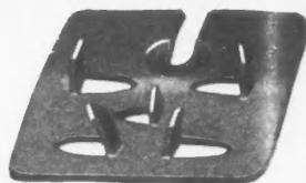
**A View of Prong Side of a Self-Clinching Fastener, Showing the Four Curved Prongs Which Clinch Into the Board, and the Straight Prong Which Holds Panel of Wallboard From Slipping to Either Side.**
