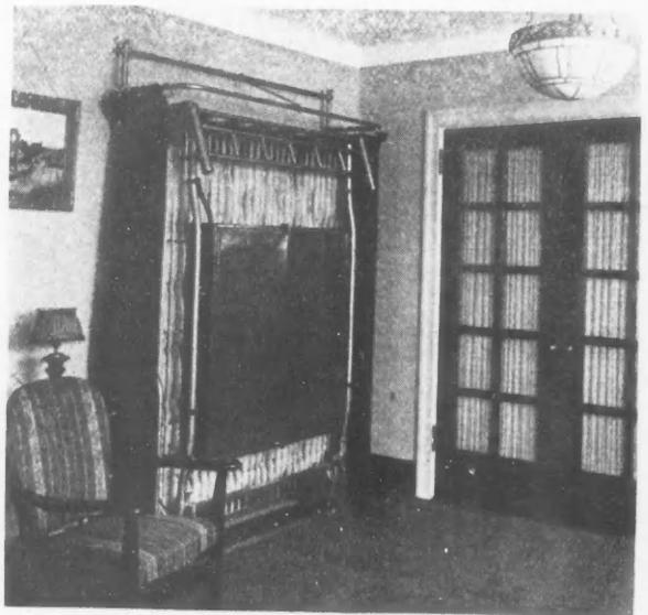
Space-Saving Wardrobe Attached to Wall Bed. It Eliminates Clothes Closet in Floor Plan.
