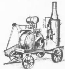
7 cu. ft. capacity, 4 H. P. engine. 5 H. P. boiler.
