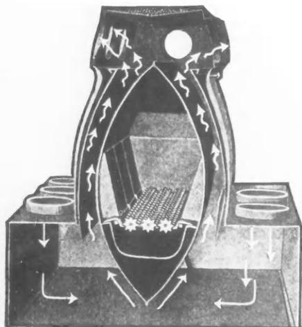
This cut shows how the FarQuar Furnace is scientifically designed to gently warm the cool, fresh air instead of rendering it lifeless and devitalized through super-heating.
