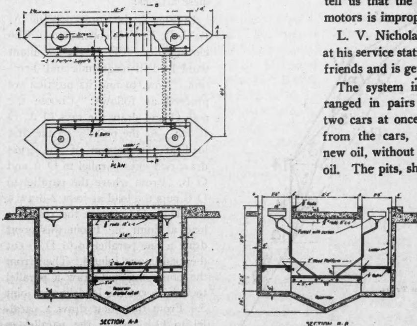
Design for Concrete Oil Draining Pits for Public Garages. These Drawings Show Cross Longitudinal Sections and Top View.
