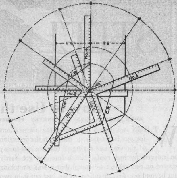
Fig. 4. Showing How Square Is Applied to Building That Is Out of Square.
