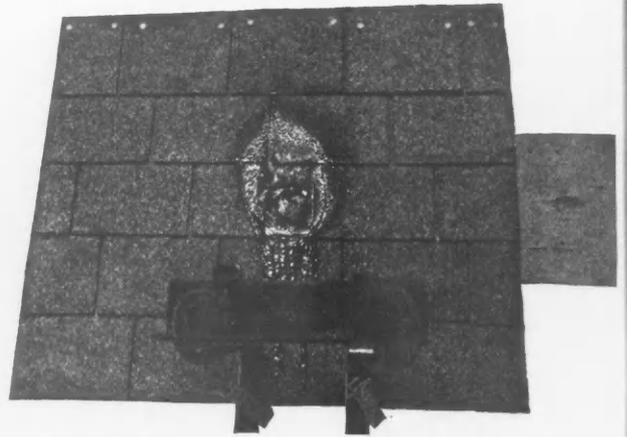
*The test was continued for 45 minutes. After the torch was extinguished, this picture was taken. The asphalt surface, at the spot where the flame struck the shingles, was somewhat melted and some of the asphalt had run, but the shingles were not burned through. The roof board was withdrawn. Small spot visible on the board was not burned nor even charred, it is merely a stain from the asphalt that softened on the underside of the shingles.*
