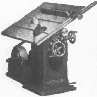
An "American" Contractors' Portable Variety Woodworker with 20-inch Band Saw.
