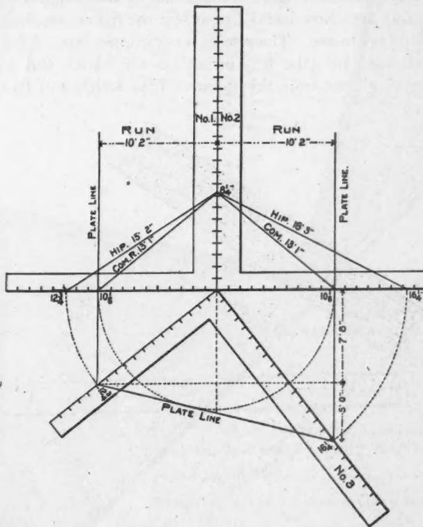
Fig. 2. Same Principle as Shown in Fig. 1. Applied to Building Out of Square.
