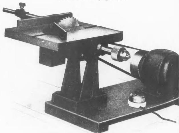
**Small Bench Machine for Light Work in Wood and Metals.**
