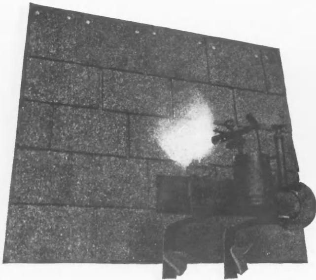
*This picture shows the test after the torch had been burning for 5 minutes.*
