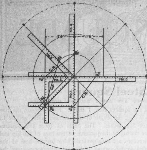
Fig. 3. Heel of Square Placed on a Center Line to Solve Problem Shown in Fig. 2.
