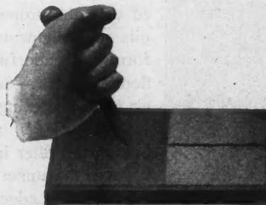
Knife Blade Test. A Test of a Cement Surface by Drawing a Knife, Spike or Other Hard Iron Instrument Over Same, Bearing Quite Heavily. The Half of the Block at the Right Is a Normally Hardened Cement Surface, Whereas the Half at the Left Has Been Hardened Chemically. Note the Difference in Depth of Scratch Caused by the Knife.
