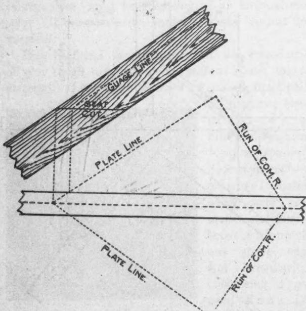
Fig. 5. Diagram Showing How to Find Backing Lines on the Hip for the Accurate Corner.
