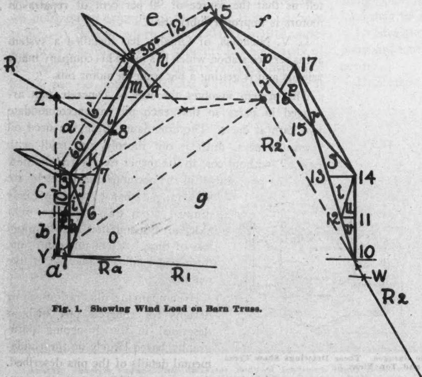
Fig. 1. Showing Wind Load on Barn Truss.
