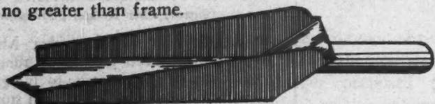
Trowel invented by Oscar Mann, Indianapolis, Ind. Especially valuable in rural section where ordinary mechanic can lay brick with the use of this tool.
