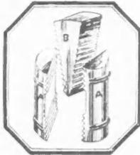
This wedge consists of three parts. The two pins (A) are inserted in a hole drilled in the end of the handle. The Tapered Wedge (B) is driven between the pins. Ordinary Wedges cannot be reset. The VAUGHAN'S EXPANSION WEDGE can be reset. Simply set the tapered Wedge (B) a notch or two deeper and a tight Handle is assured.
