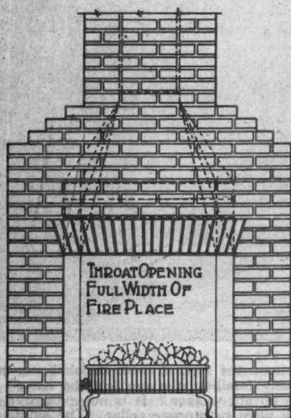
Fig. 1. Dotted lines show how fireplaces should not be built. Side walls should not be drawn in below the top horizontal dotted line. This assures full area.
