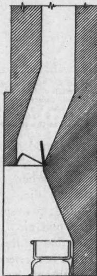
Fig. 4. Wrong Location for Throat Damper. The Throat is so Low That the Accumulation of Gases at the Point Constricted Weakens the Draft with Greater Likelihood of a Smoky Fireplace. The Smoke Shelf is Bricked Up, Which is Wrong.
