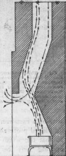
Fig. 3. Fireplaces Constructed Like This Without Throat will Very Likely Smoke.
