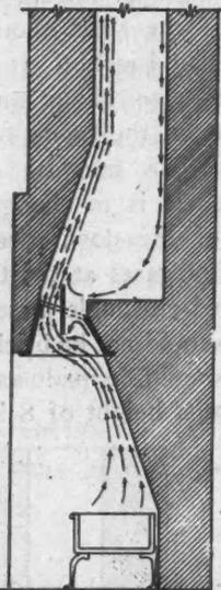
Fig. 6. Smoke Dampers with Lids Hinged in the Center do Not Turn the Up Draft as Well as Do Those Hinged at the Rear Side.
