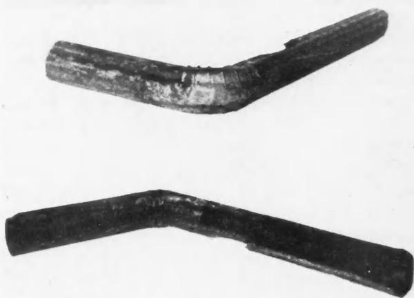
Fig. 2. Elbow and Down Spouting Subjected to Same Conditions for Three Years. The Elbow, Which Is Pure Iron, Has Shown Greater Resistive Powers Than the Common Steel.
