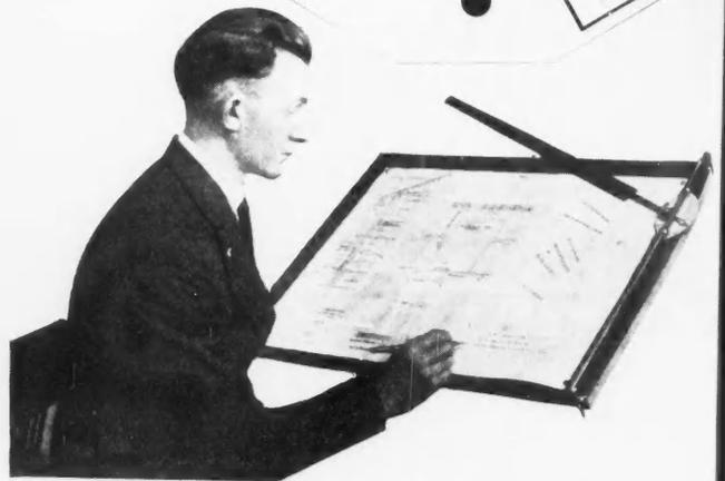
**New Device Is Attachable to Any Side of the Drawing Board and Is Useful for Charting, Plotting and Drafting Generally. Above, the Method of Using It to Determine Roof Pitches.**
