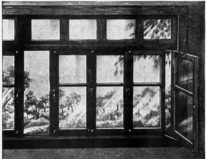
Showing how the AiR-Way link opens each window. In each series of sash, the sash hinged to the window casing opens first. Then the remaining sash slide toward this end as they are opened.
