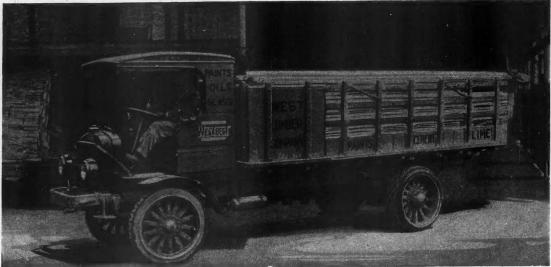
4-CYLINDER, 4 TO 6 TON AUTOCAR; 156 INCH WHEELBASE; CHASSIS PRICE \$4800
