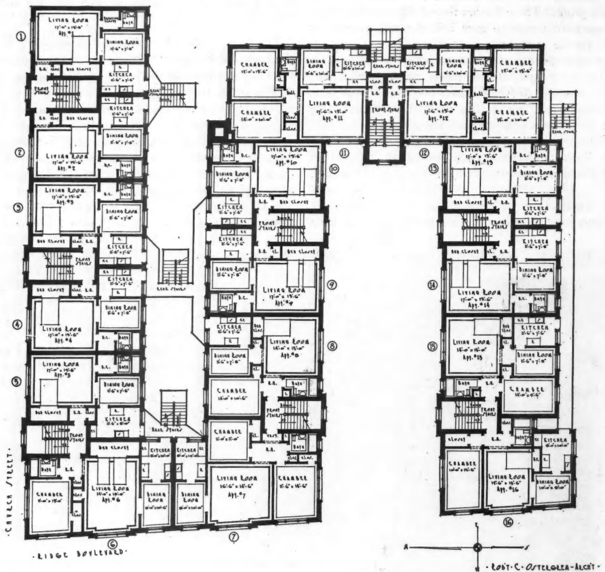
Typical Floor Plan of the Andridge Co-Operative Apartments as Illustrated on Page 114. Notice the ample provision for light and air. Every room is an outside room.
