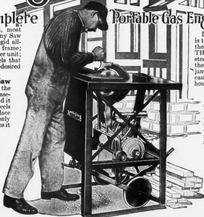
Its distinguishing feature is the saw, which operates on the swing method—moving THROUGH the lumber instead of the lumber through the saw. Quicker, easier; no jamming of the blade. Starts easily. Runs smoothly; 10 hours on 1 gallon of gasoline.
