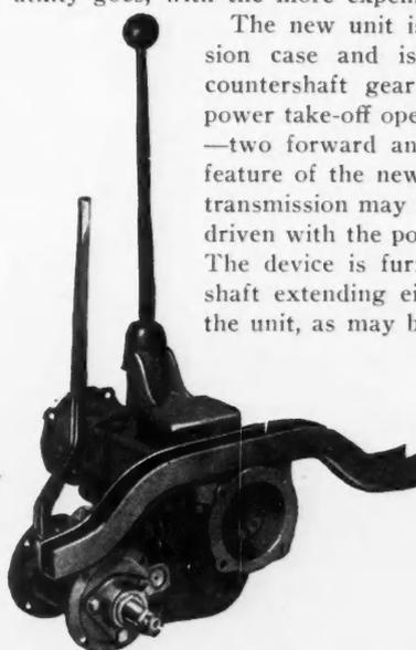
This Power Take-Off Can Be Used Effectively in Combination with a Six-Speed Auxiliary Transmission.
