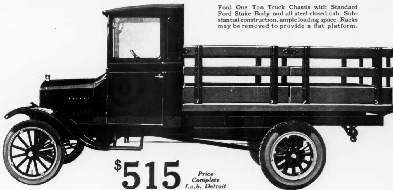
Ford One Ton Truck Chassis with Standard Ford Stake Body and all steel closed cab. Substantial construction, ample loading space. Racks may be removed to provide a flat platform.
