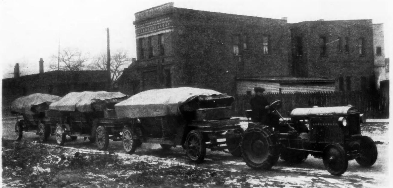
Equipment Like This Will Replace Four Teams of Horses and Do the Work More Quickly and More Cheaply. Recently the use of tractors has displaced horses not only for heavy hauling of this type but also for the short haul where time is consumed in loading and unloading. The tractor can be kept in constant operation while its trailers are taking on their loads or dropping them at the destination.
