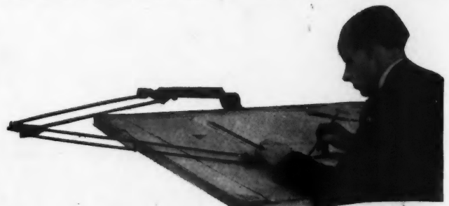
Much Time Can Be Saved in the Drafting Room by the Adoption of This Device Which Is Attached to the Drafting Table to Save Mechanical Drudgery.
