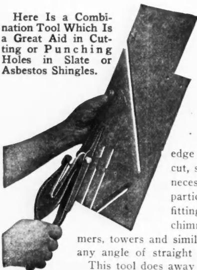
Here Is a Combination Tool Which Is a Great Aid in Cutting or Punching Holes in Slate or Asbestos Shingles.
