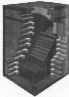
The Step-Like Grate of This Incinerator Is a Feature Which Greatly Improves Combustion.
