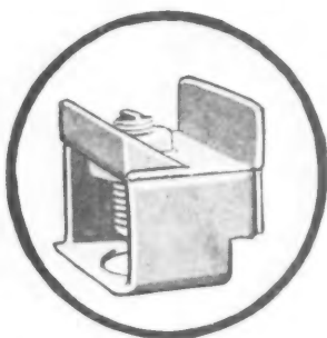
The Reinforcing Bracket, a heavy, rigid brace, prevents distortion during setting. It supports the copper gutter as the indirect pressure of the Zouri Key draws the moulding into alignment
