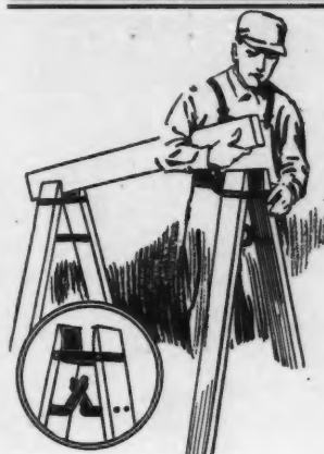
Close-Up Showing How Steel Jaw Grips Cross Member.
