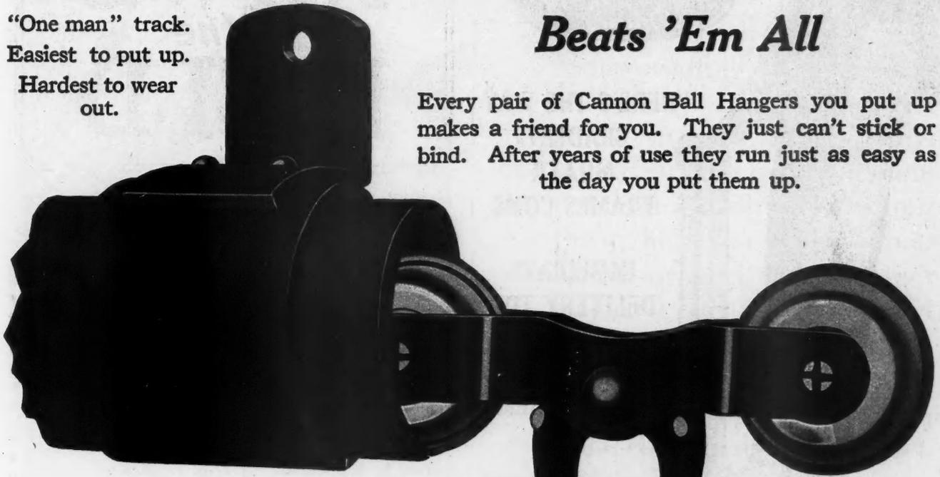
No. 1068 Hanger illustrated here has pressed steel ball wheels, enclosed in a round track shielded from weather. The slot is at the very bottom of the track so that condensed moisture runs out and does not mingle with rust, scale and dirt to freeze and stop the hangers. Adjustable three ways—for thin or thick doors—for movement up or down—to or away from building.
