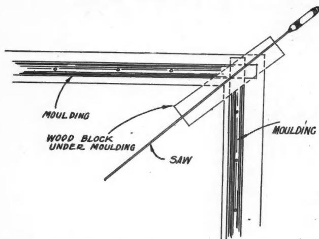
The Screen Wire Moulding Will Fit Perfectly if Cut in This Way and It Saves Time, Too.
