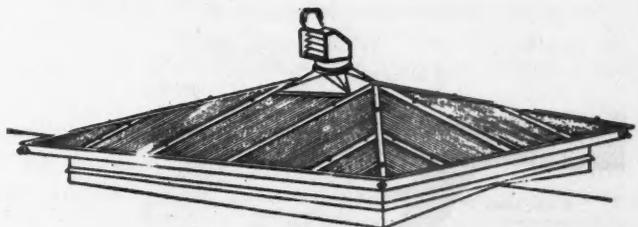
Here Is a Mechanically Constructed Skylight Which Is Easily and Quickly Installed Because There Is Nothing to Be Cut or Fitted.
