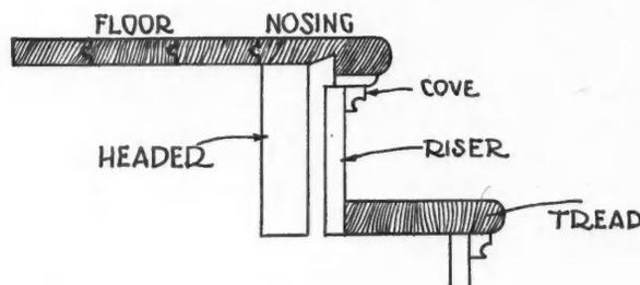
A Quick Way to Provide Nosing When Ready Cut Nosing Is Not Available.
