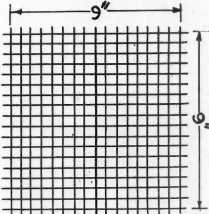
A Piece of  $\frac{1}{2}$ -Inch Mesh Wire Cloth Makes an Excellent Scratcher for Stucco.
