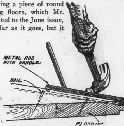
A Short Handle Is a Real Improvement of the Steel Piece Suggested for Laying Flooring.
