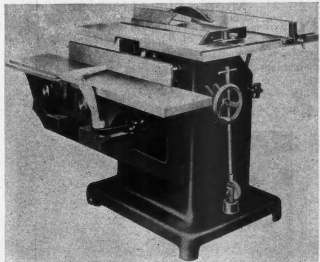
**Here Is a Combination Saw and Jointer Made Up of the Standard Units Manufactured by a Leading Company in This Field.**
