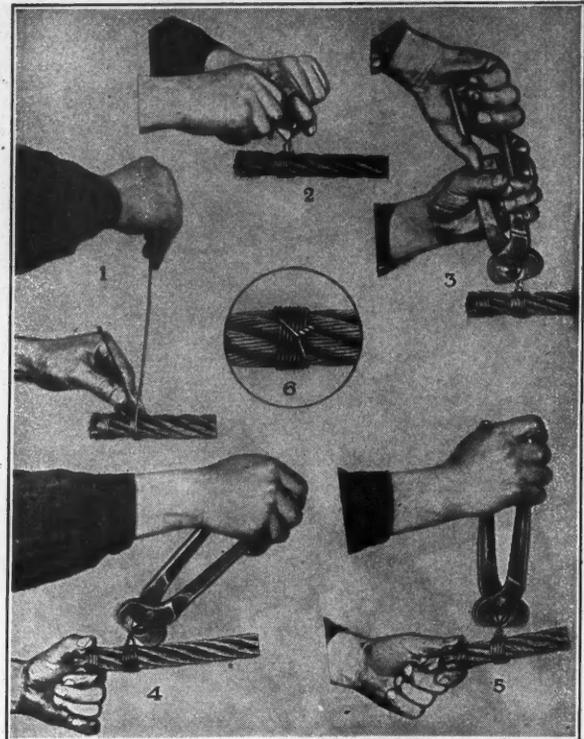
Illustrated Here Is the Proper Method for Seizing Wire Rope.
