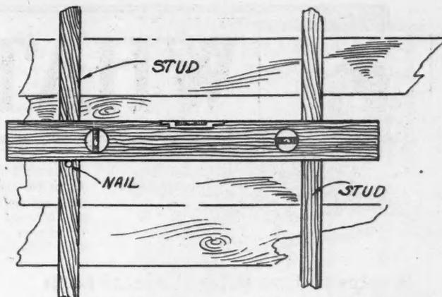
This Method of Testing a Level Is Simple and Exact.
