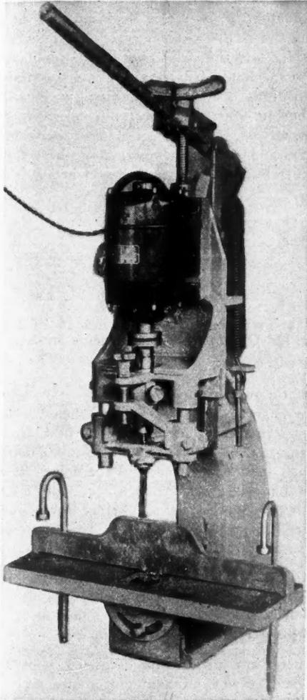
Here Is a Mortiser Designed to Be Either Mounted on a Bench or on a Truck with Casters to Move About the Shop.
