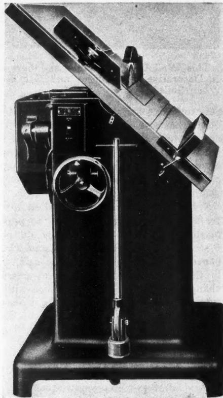
This Motor on Arbor Machine, Operating from the Lighting Circuit, Incorporates Many Improvements.
