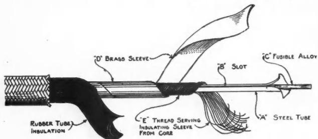
The Heart of the Fire Detecting System Is This Fire Detecting Wire with a Core of Fusible Alloy Sensitive to "Fire Conditions."
