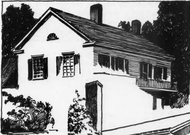
FIG. 4. THE RAILED DECK IS ONE OF THE MOST COMMON ATTACHMENTS SEEN ON THE COLONIAL OF LATER DATE. NO LOWER PORCH IS USED NOR ARE THERE ANY SUPPORTING COLUMNS.
