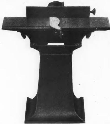
A guard is provided which assures perfect safety and the machine is notably easy to operate. It is provided with a three-knife cutter head, a long table and tilting fence. The cutter head is 6 3/4 inches wide and the table measures 33 by 8 inches. The height of of the table when used with the base, is 33 inches, but the machine is also available as a bench machine. It operates at a speed of 3,600 R.P.M.
