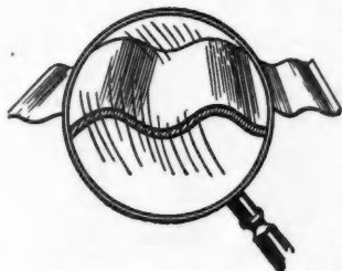
Two surfaces of Pure Lead seal a core of special analysis, copper content steel.
