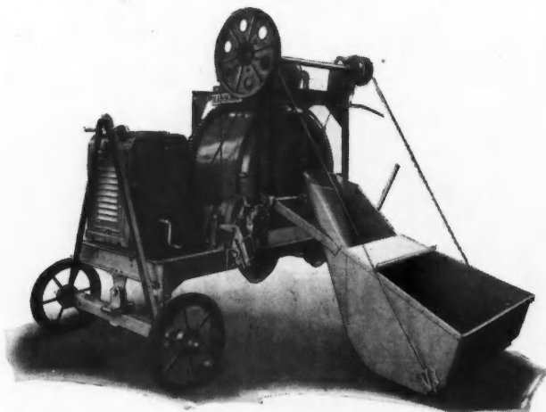
A Standard, One Bag, Building Mixer Which Has Recently Been Added to a Well Known Line Is a Quality Product.
