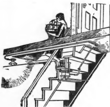
Automatic Control of Basement, Attic or Other Lights with a Switch in the Stair Tread.
