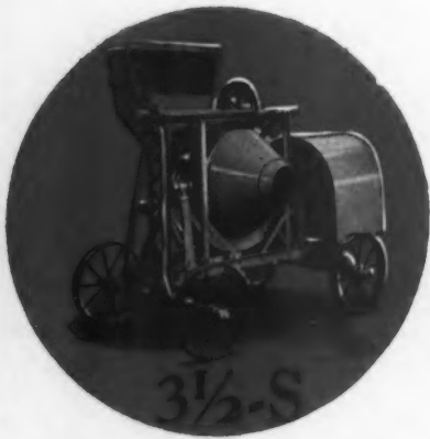
Smith 3 1/2-S Tilter — another mixer of 8 seconds discharge—furnished with or without power loader. Can be had as two-wheel trailer or with 4 steel or cushion-tired wheels. Capacity 35 to 50 yds. a day.
