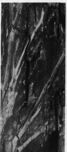
11-Water-Conducting Strands Fig. 11—Water-Conducting Strands on the Underside of the Pine Flooring, Laid Over Brick, Shown in Figure 3.
