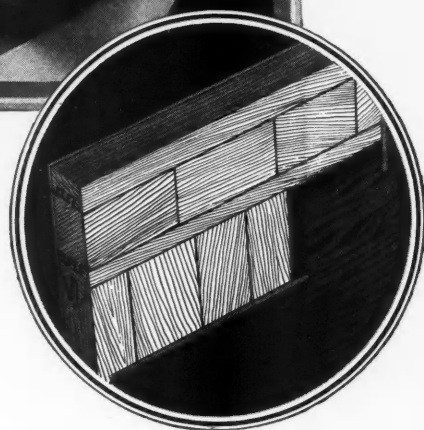
The Laminex stile is built of separate core blocks with crossed grains. Any tendency of the one to shrink or swell is counteracted by an opposing tendency of its neighbor. Blocks are locked together and dovetailed to full-length edge braces with water-proof Laminex cement.
