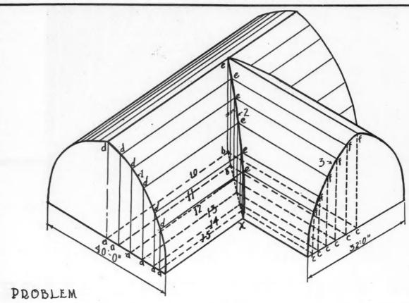
To Layout The Rafters of a Gothic Roof With an addition - The Main Part is 40'-0" Wide and The Radius is 28'-0". The Point of Radius is on The Base Line. The Addition is 32'0" Wide, But The Height is The Same.
