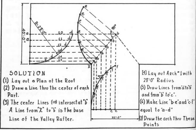
Here Is Illustrated the Solution of a Problem in Framing Gothic Roof, as Discussed on Page 100. The upper drawing shows the reasoning for the steps shown below.
