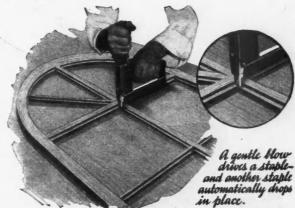
A Machine Which Makes for Economy in Tacking the Light Frames in Making French Doors.
