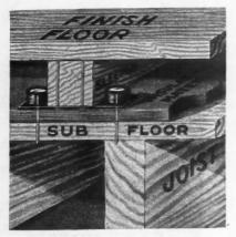
With This Clip in Use the Finished Floor "Floats" on Insulating Material.
