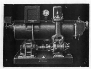
Independent Air and Water Units Are Compactly Built Into This Vacuum Heating Pump, Saving Expense in
