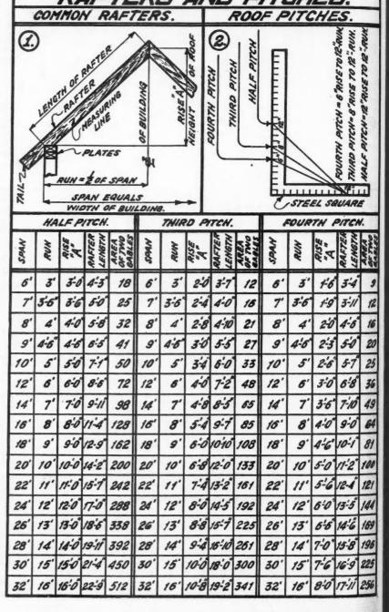
Figs. 1 and 2. Showing the Various Measurements of Common Rafters and the Roof Pitches in the Steel Square with, Below, a Table of Roof Pitches.
