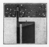
STEEL WINDOW INSERTS are formed strips of galvanized rust-resisting Armco Ingot iron which provide recesses in jambs and across openings where steel windows are to be used. Two types—one for concrete construction and finish and another for buildings of concrete frame faced with brick.
