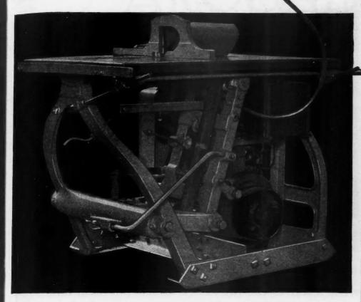
In 2 Sizes: No. 3 and No. 5 Tilting Table Straight-Line Cut-Off Cut-Under Frame Radiator-Cooled Engine Engine Under Table Efficient Saw-Guards Hand or Foot Operation Easily Adjustable Gauges Adjustable Arbor Shaft Self-Oiling Arbor Bearings
