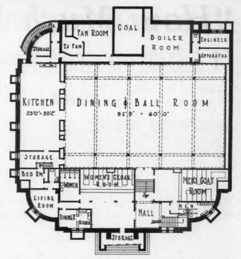
The Basement of This Building Contains, in Addition to the Heating Equipment, a Combination Dining and Ball Room and the Accompanying Coat Rooms.
