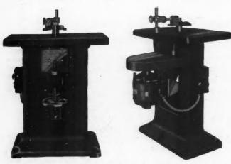
Two Views of a New, Single Spindle Shaper Designed for Accurate Work, with a Heavy Frame to Eliminate Vibration.
