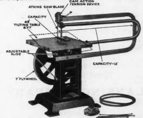
This "Up-to-Date" Superior Jig Saw, complete with Blades, Belt and Pulley, only \$15.00. It has a sawing capacity of 12", will handle 1" stock, has a 7" fly-wheel, and a tilting saw table 6"x7". Made of the best materials and fully guaranteed. Write for full details.
