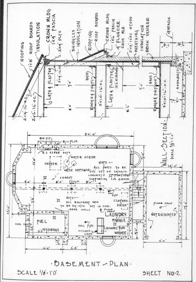
In the Basement of the Modern Home Will Be Found Some of the Most Important Items of Equipment, While Other Specialties Enter Into the General Construction as Indicated in the Wall Section.
