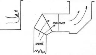
Fig. 1—The Incorrect Method (Left) and the Correct Method (Right) of Making a Transition from an Oval Riser to a Floor Register in Warm Air Heating.
