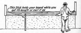
A Small Stick Tacked to the Center of a Long Piece of Trim Takes the Place of a Helper When Working Alone.
