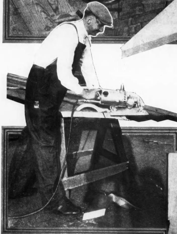
Above: By Means of the Tilting Base, Set at a 45 Degree Angle, It Is Possible to Cut a Number of Hip Jack Rafters Requiring the Compound Miter Cut, Without Changing the Angle of the Base.
