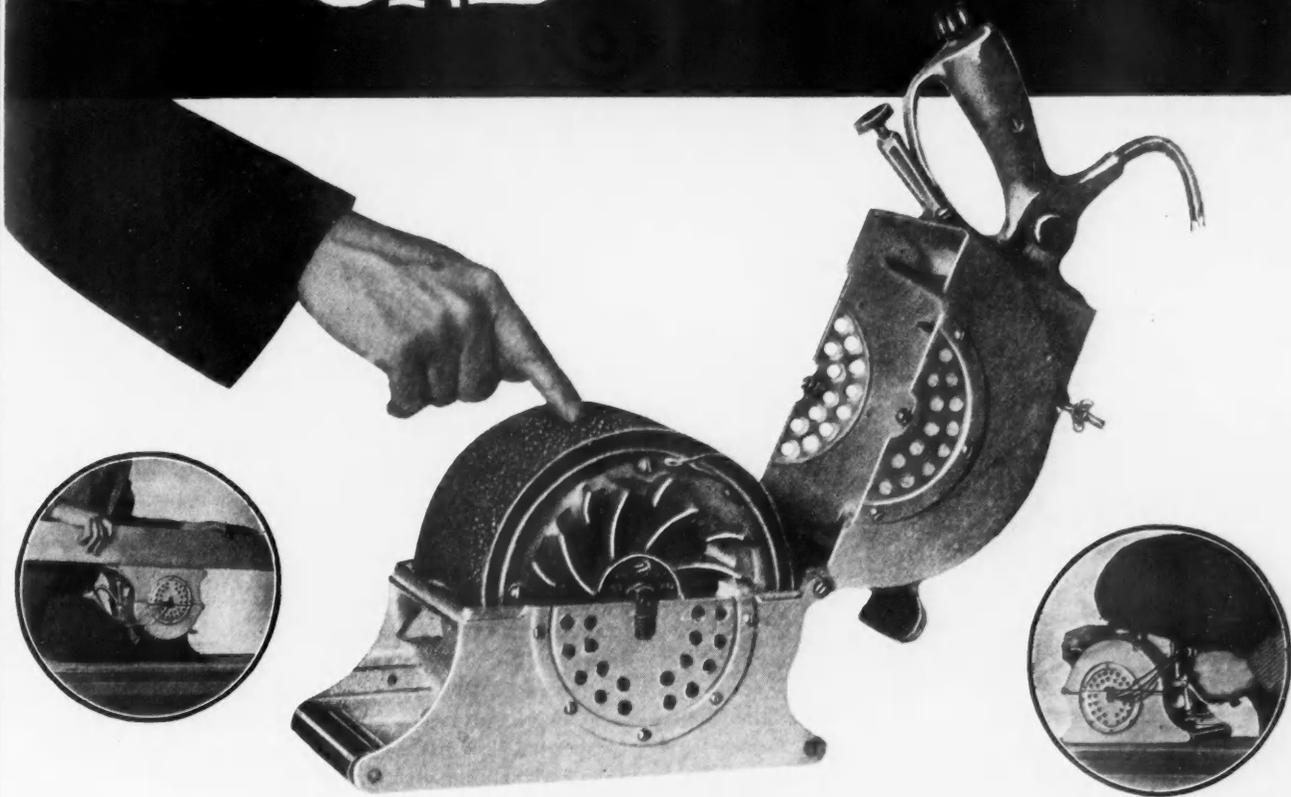
Before the Reid-Way came on the market, it was thought necessary to drive sanding drums through belts, chains or gears. This meant added weight and loss of power. The Reid-Way revolving field motor brought a new conception of a light weight sanding machine. The sanding drum itself is the motor and this high-speed, high-efficiency, sander with remarkably long life has won nation-wide recognition.
