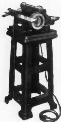
This oilstone grinder is equipped with  $\frac{1}{2}$  h. p. motor. There are no belts in the construction, the motor being directly connected. The oilstone wheels are geared for the proper speed.
