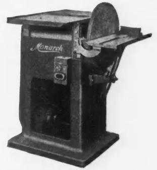
**Ball Bearing Drum and Disc Sander**—Requires minimum power and attention. Completely adjustable drum shaft, outside of main frame. Write for prices.
