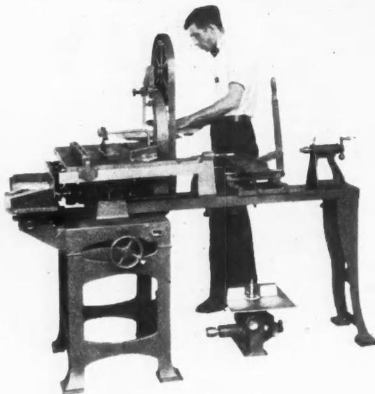
Eight Woodworking Machines in One, the Units of Which Can Be Purchased Separately and Added as Needed.
