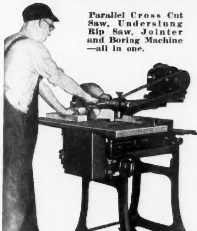
Parallel Cross Cut Saw, Underslung Rip Saw, Jointer and Boring Machine—all in one.
