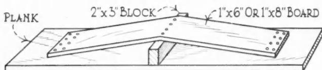
A Weak Scaffold Plank Braced Like This Is Perfectly Safe But Should Be Tested Before Using.
