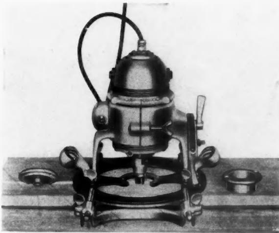
A Tilting Base for the Router Increases Its Efficiency and at the Same Time, Reduces the Cost of Operation.
