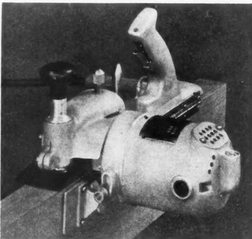
Just As the Electric Saw Has Replaced the Hand Saw, So the Electric Plane is Replacing the Hand Plane for Fitting Doors.
