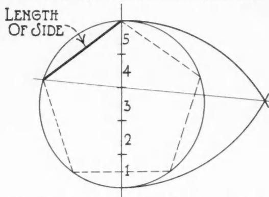
Any Polygon Can Be Laid Out Accurately by This Method If It Is Done Carefully.
