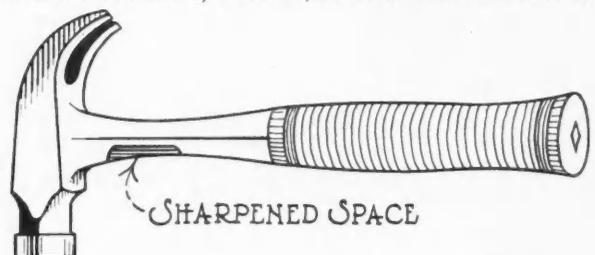
Sharpened as Shown This Hammer is a Handy Tool to Use When Applying Wood Shingles.
