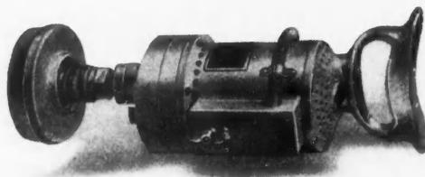
Much Tedious Labor Formerly Used in Smoothing Concrete Is Saved When An Electric Surfer Is Employed.
