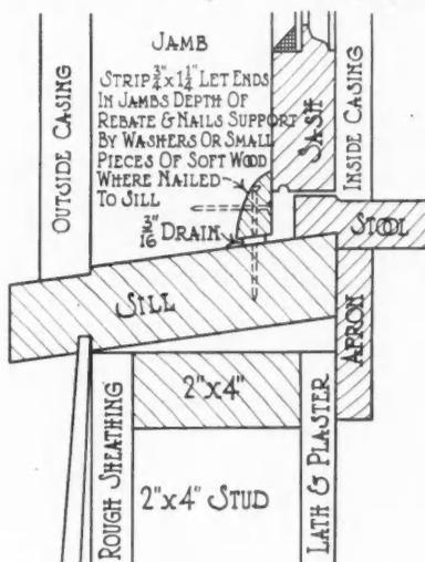
This Construction Prevents Leakage Around Casements.
