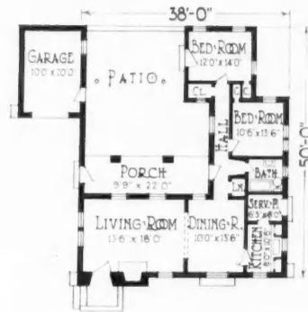
Although Small, This House of Unique Old Pueblo Design Has a Large Amount of Living Capacity. The selling price with lot was \$5,385. Walls are of adobe construction with brown stucco. Designed and built by John W. Murphey Building Co.
