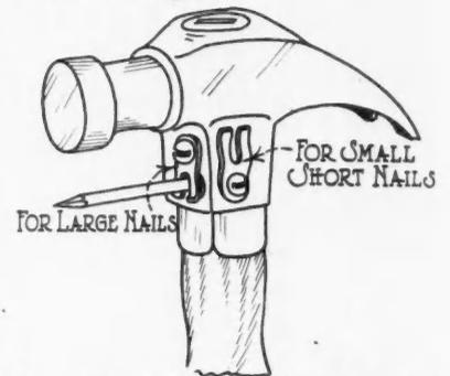
The nail is held firmly in the clip, in the correct position to start it with one blow. Then the hammer is pulled releasing the nail from the clip. You can then go ahead and drive the nail.
