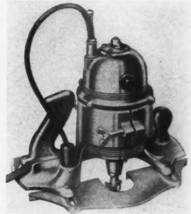
Grooving Flooring After It Is Laid Can Be Done Speedily and Accurately with This Power Tool.
