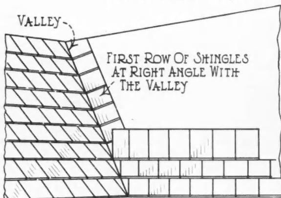
You Can Save Cutting Shingles by Using This Method of Shingling the Valley.
