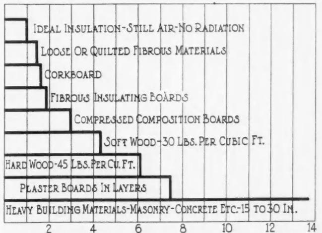
Figure 1. Thickness of Various Materials Having Equivalent Heat-Insulating Values. The Number of Inches for Each Material Shows the Thickness Required to Equal One Inch of Ideal Insulation.
