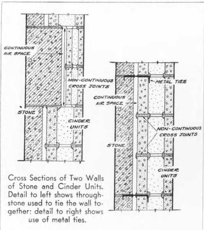
Cross Sections of Two Walls of Stone and Cinder Units. Detail to left shows through-stone used to tie the wall together; detail to right shows use of metal ties.
