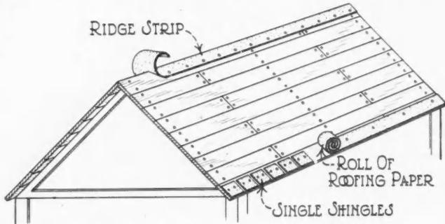
Roll Roofing Used at Eaves and Ridge with Asphalt Shingles Save Time and Makes a Better Job. Sketch shows comparison.
