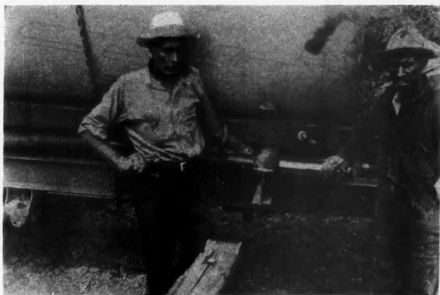
A Frame Attached to the Truck Chassis for Hauling Heavy Pipe.
