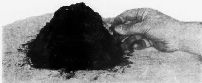
Two quarts of dirt are removed each month from the air admitted to the Proving House; oil treated steel wool filters are used. It is not unusual for this amount of dirt to be found in the air circulated through average high grade residential buildings . . .
