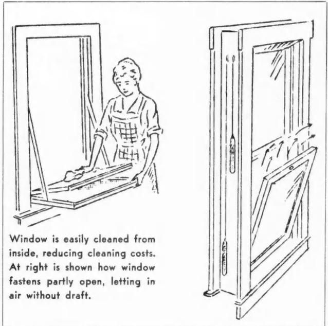
Window is easily cleaned from inside, reducing cleaning costs. At right is shown how window fastens partly open, letting in air without draft.
