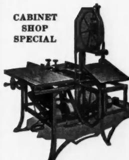
Includes 16" hand saw, 6" jointer and 8" circular rip and crosscut saw. Without Motor \$247
