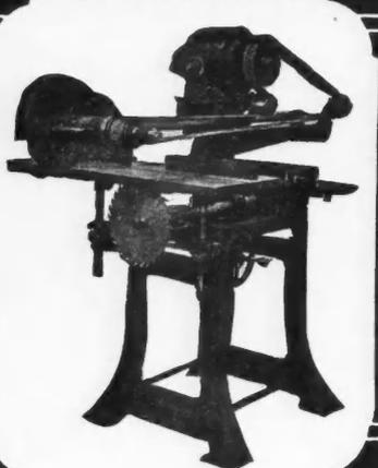
This remarkable machine cuts costs as quickly and as surely as it cuts wood! Does the work of five ordinary machines—eighteen different everyday jobs—faster and at less cost! Cross-cut saw, rip saw, jointer, shaper and router—five machines in one . . . at the cost of one. Ball-bearing throughout. Write for full particulars.
