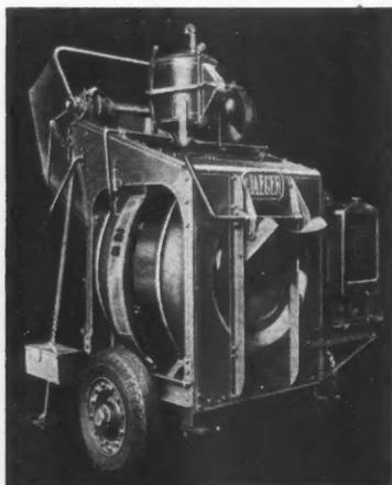
Streamlined tilting mixers are offered in 3½S to 7S sizes, featuring the Jaeger patented "Dual Mix" drum with "V" bottom on all models, a pneumatic tired 3½S trailer, and a popular priced 5S size with 2-wheel trailer mounting and end discharge adapted for work in congested streets, backing up to cellar windows and foundations, and pouring with swinging spout.
