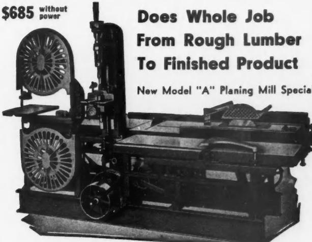
Each of these eight full-sized machines is independently operated, with all bearings high-grade ball bearings. Sturdy, compact, with no excess weight. Can be purchased on the FHA Plan—three years to pay.
