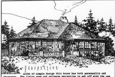
Save this house has both personality and character. The living room and entrance projection is set off with the use of Redwood board and battens with Redwood shingle or shake background. A Redwood thatched shingle roof will conform with hipped construction.
