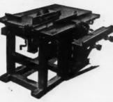
Four machines in one and so constructed that four men may use it at one time. Combines rip and cut-off saw bench with boring attachment, hollow chisel mortiser and 8" jointer. With electric motor, gasoline engine or furnished power.
